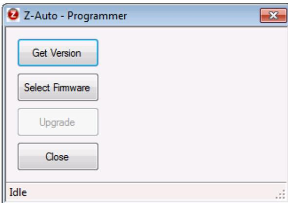
Occasionally the firmware to fail to load. You can click Upgrade again to try again. If the unit is unresponsive or all else fails, the firmware can be “force upgraded” with the following procedure:
