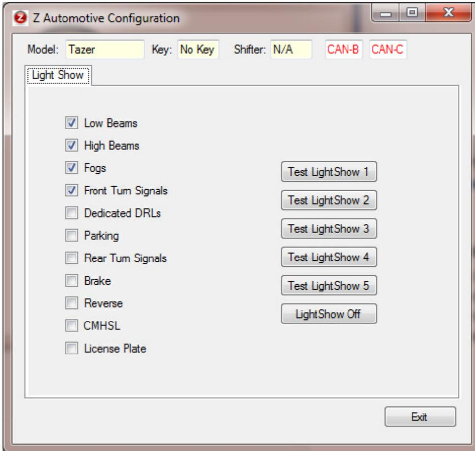
Each checkbox allows you to add or remove each light from the light shows. If connected to a car, you can try the light shows right from the ZPU screen.
