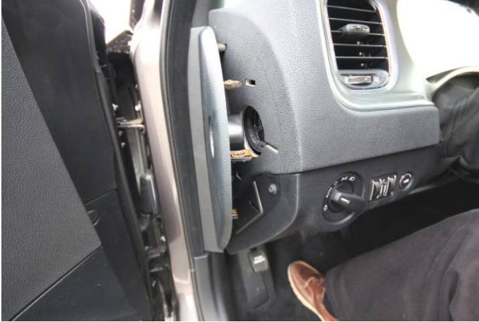
Removal of side panel; pulls off.
