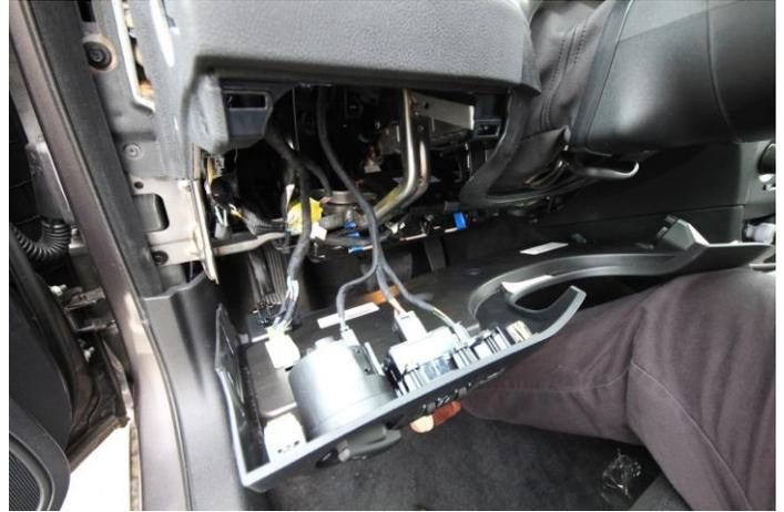
Remove 2 screws; pull lower cover straight back.
