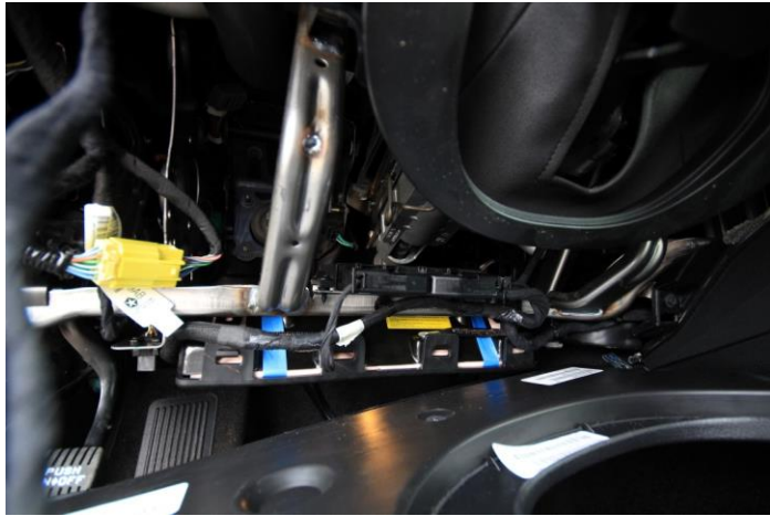
TCM located under steering column.
